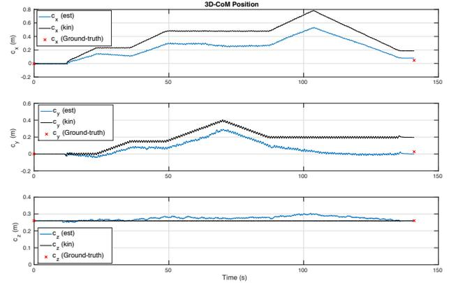
**Figure 2:** 3-D CoM trajectory, the blue lines indicate the estimated trajectories while the black lines indicate the kinematically computed ones.
