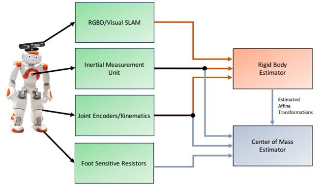
**Figure 1:** A cascade state estimation scheme that utilizes two EKFs, fusing effectively four different sensing sources, namely RGBD, IMU, joint encoders, and FSRs.
